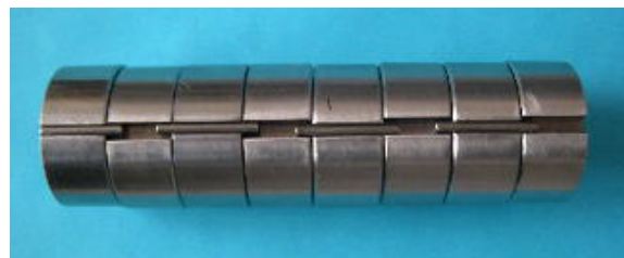
Picture 3: Assembly of eight (8) SMN mixing elements
