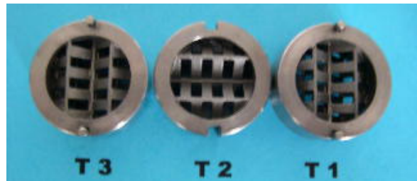
Picture 2: Orientation of slots and pins of the mixing elements T1, T2 and T3 relative to the mixer grid
