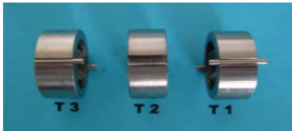
Picture 1: Three types of mixing elements: T1, T2 and T3
